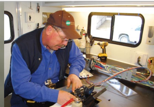
(Center) Switches for the VZW project are programmed in the lab before being deployed (Right) Splicing fiber
